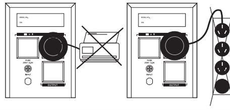
Enable the UPS by turning on the Power ON/OFF switch, which is situated on the front panel.
